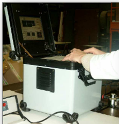
Example of device of measurement of depth of nitriding of bearing
